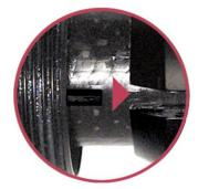
If a user opens the hand nut more than 5 turns then the pin can come out of its location in the ring. Then when the screw lock is retightened the pin may move away from its slot and will be bent or broken by the compression ring, which will be also be scored.
