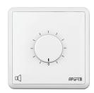
The Apart E-VOL20 is a 100 volt volume control. It can handle up to 20 watts of power and is very durable thanks to the step-by-step attenuation in 11 steps + zero position. The E-VOL20 is designed to handle 24V priority signals. This means that you can always get an announcement out, even to zones where the local volume control is in the 'OFF' position!
