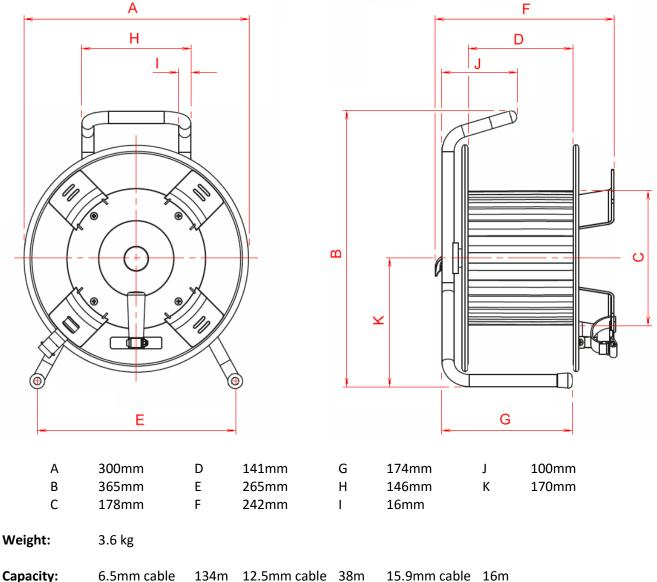
Capacity: 6.5mm cable 134m 12.5mm cable 38m 15.9mm cable 16m For more capacities use the online cable drum calculator <u>http://www.canford.co.uk/Technical/Article/CableDrumCalculator?portable=true</u>
