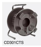
Robust cable-drum, steel drum with steel tube frame. Friction drum-brake incorporated into the frame to prevent movement in transit. 'Cable tail' type drum with solid steel flange open hub plus four brackets on the flange face to enable the cable tail to be brought out from the hub of the drum at a gentle angle (important for coaxial and essential for fibre cables) and coiled and secured around the brackets.. Fixed handle. Black finish.
