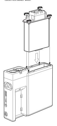
**2** Fasten four mounting screws of the receiver/tuner unit with a screwdriver.
