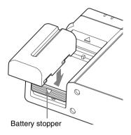
2 Slide the battery into the compartment while maintaining its horizontal orientation until the battery stopper returns to its original position.
