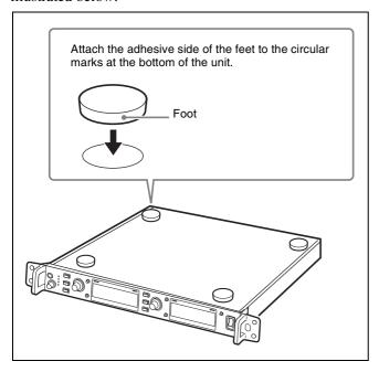
To install the DWR-R02DN in the rack, be sure to remove the attached feet.
