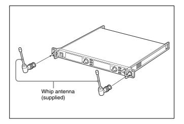
**3** Use commercially available BNC cables (50  $\Omega$ , 60 cm or longer) to connect the antenna mounts with BNC connectors to the ANTENNA a/b IN connectors on the rear panel of the unit.
